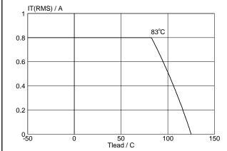
Fig.3. Maximum permissible rms current  $I_{T(RMS)}$ , versus lead temperature, T<sub>lead</sub>.
