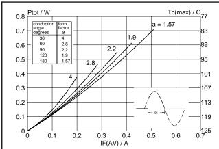
Fig.1. Maximum on-state dissipation,  $P_{tov}$  versus average on-state current,  $I_{T(AV)}$ , where  $a = form \ factor = I_{T(RMS)} / I_{T(AV)}$ .
