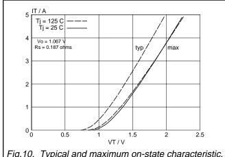
Fig.10. Typical and maximum on-state characteristic.
