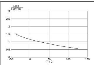
Fig.8. Normalised latching current  $I_L(T_j)/I_L(25^{\circ}C)$ , versus junction temperature  $T_j$ ,  $R_{GK}=1$  k $\Omega$ .
