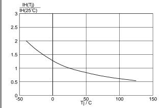
Fig.9. Normalised holding current  $I_H(T_j)/I_H(25^{\circ}C)$ , versus junction temperature  $T_j$ ,  $R_{GK}=1$  k $\Omega$ .
