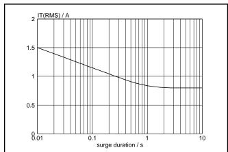
Fig.5. Maximum permissible repetitive rms on-state current  $I_{T(RMS)}$ , versus surge duration, for sinusoidal currents, f = 50 Hz;  $T_{lead} \le 83$  °C.
