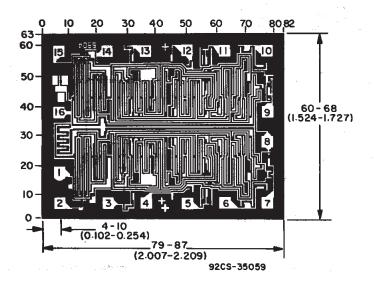
Dimensions in millimeters are derived from the basic inch dimensions as indicated. Grid graduations are in mils ( $10^{-3}$ ).
