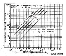
Fig.6 - Typical power dissipation vs. frequency.
