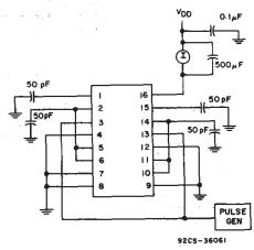
Fig. 13—Dynamic power dissipation test circuit.
