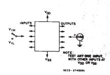
Fig.8 - Input-voltage test circuit.
