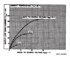
Fig.2 — Typical output low (sink) current characteristics.
