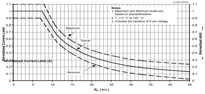
Figure 35. Normalized Current Limit vs. External Current Limit Resistance.
