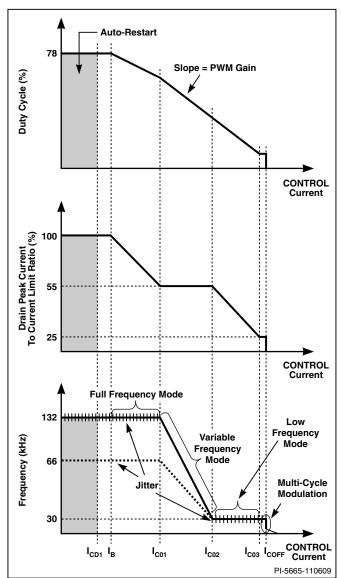
Figure 5. Control Pin Characteristics (Multi-Mode Operation).
