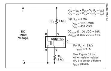
Figure 22. Line Sensing and Externally Set Current Limit.
