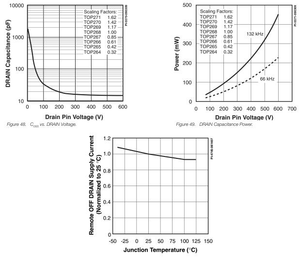
Figure 50. Remote OFF DRAIN Supply Current vs. Temperature.
