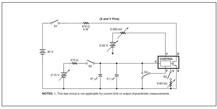
Figure 33. TOPSwitch-JX General Test Circuit.
