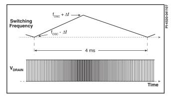
Figure 6. Switching Frequency Jitter (Idealized V<sub>DRAIN</sub> Waveforms).
