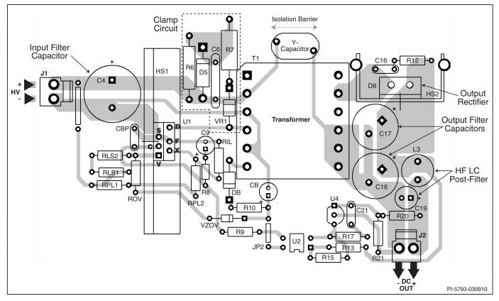
Figure 29. Layout Considerations for TOPSwitch-JX Using E-Package and Operating at 132 kHz.
