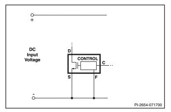
Figure 10. Full Frequency Operation (132 kHz).
