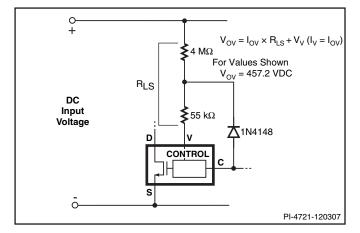
Figure 16. Line-Sensing for Overvoltage Only (Undervoltage Disabled). Maximum Duty Cycle Reduced at Low Line and Further Reduction with Increasing Line Voltage.
