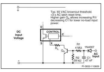
Figure 23. Externally Set Current Limit, Fast AC Latch Reset and Brownout.
