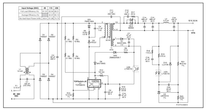
Figure 25. Schematic of High Efficiency 12 V, 30 W, Universal Input Flyback Supply With Very Low No-load.
