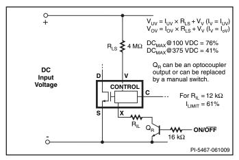
Figure 21. Active-on Remote ON/OFF with Line Sense and External Current Limit, and Latch Reset.
