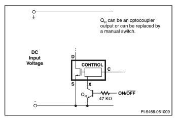
Figure 19. Active-on (Fail Safe) Remote ON/OFF, and Latch Reset.
