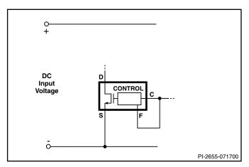
Figure 11. Half Frequency Operation (66 kHz).
