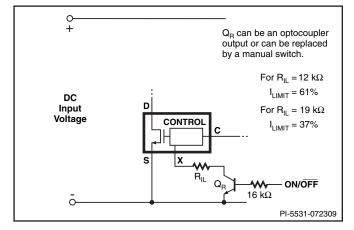
Figure 20. Active-on Remote ON/OFF with Externally Set Current Limit, and Latch Reset
