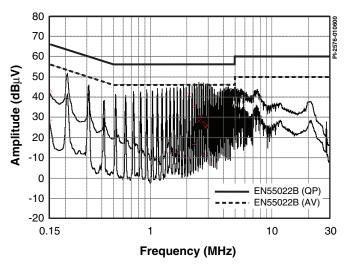
Figure 26. Fixed Frequency Operation Without Jitter.
