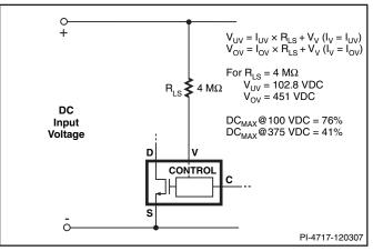
Figure 13. Line-Sensing for Undervoltage, Overvoltage and Line Feed-Forward.
