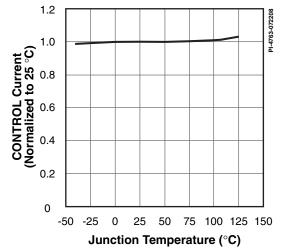
Figure 44. Control Current Out at 0% Duty Cycle vs. Temperature.
