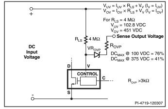
Figure 14. Line-Sensing for Undervoltage, Overvoltage, Line Feed-Forward and Hysteretic Output Overvoltage Protection.
