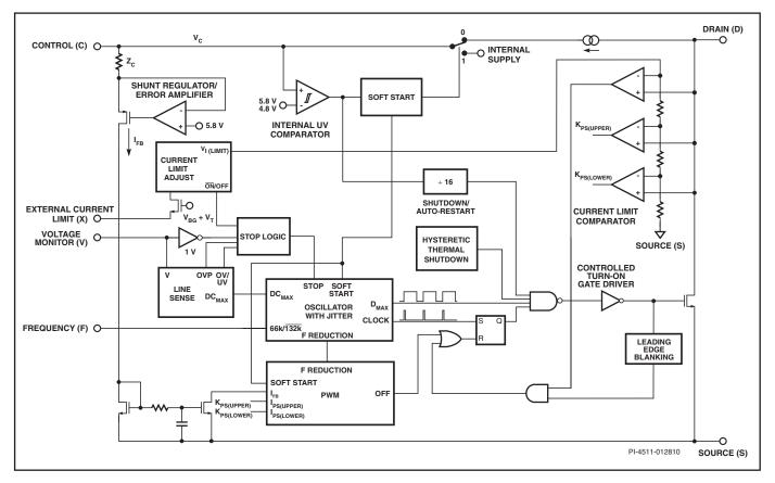
Figure 2. Functional Block Diagram (E and V Package).
