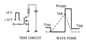
$$R_{G} = 25~\Omega,~V_{DD} = 90~V$$
