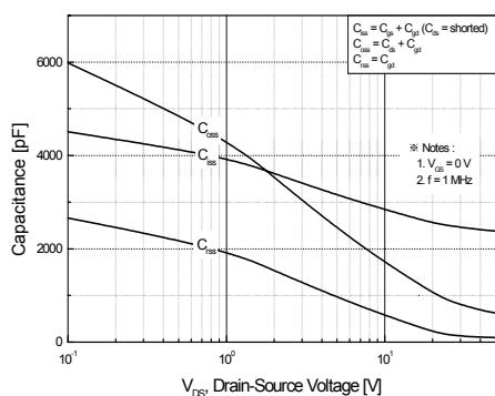
**Figure 5. Capacitance Characteristics**
