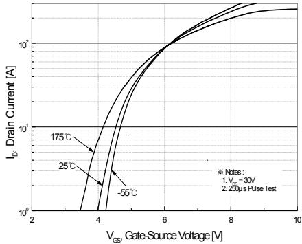
**Figure 2. Transfer Characteristics**
