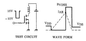
$R_G = 25\Omega$  $V_{DD} = -50V$ , L=1.44mH  $E_{AS} = \frac{1}{2} \cdot L \cdot I^2 \cdot (\frac{B_{VDSS}}{B_{VDSS} - V_{DD}})$
