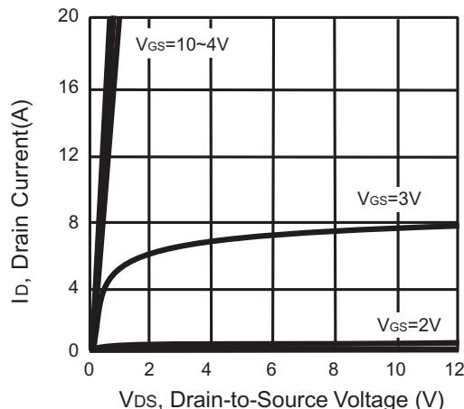
Figure 1. Output Characteristics
