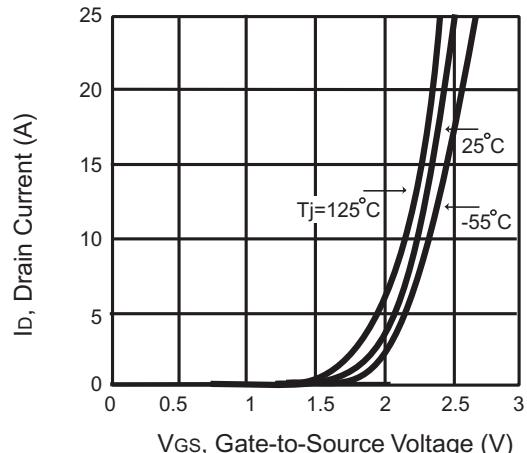
Figure 2. Transfer Characteristics
