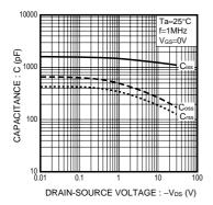
Fig.7 Typical Capacitance vs. Drain-Source Voltage
