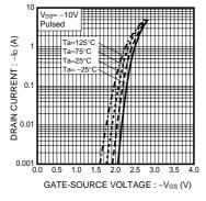
Fig.1 Typical Transfer Characteristics
