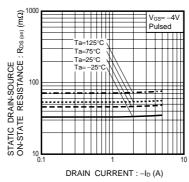
Fig.5 Static Drain-Source On-State vs. Drain Current
