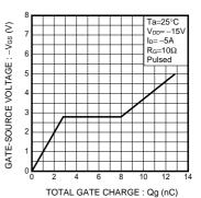
Fig.9 Dynamic Input Characteristics
