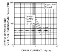
Fig.4 Static Drain-Source On-State vs. Drain Current
