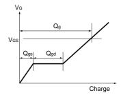
Fig.13 Gate Charge Waveform
