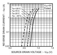
Fig.6 Reverse Drain Current Source-Drain Current
