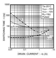
Fig.8 Switching Characteristics
