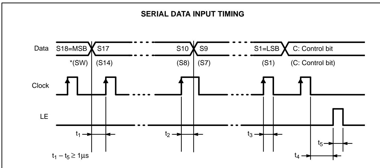
On the rising edge of the clock shifts one bit of the data into the shift registers.
