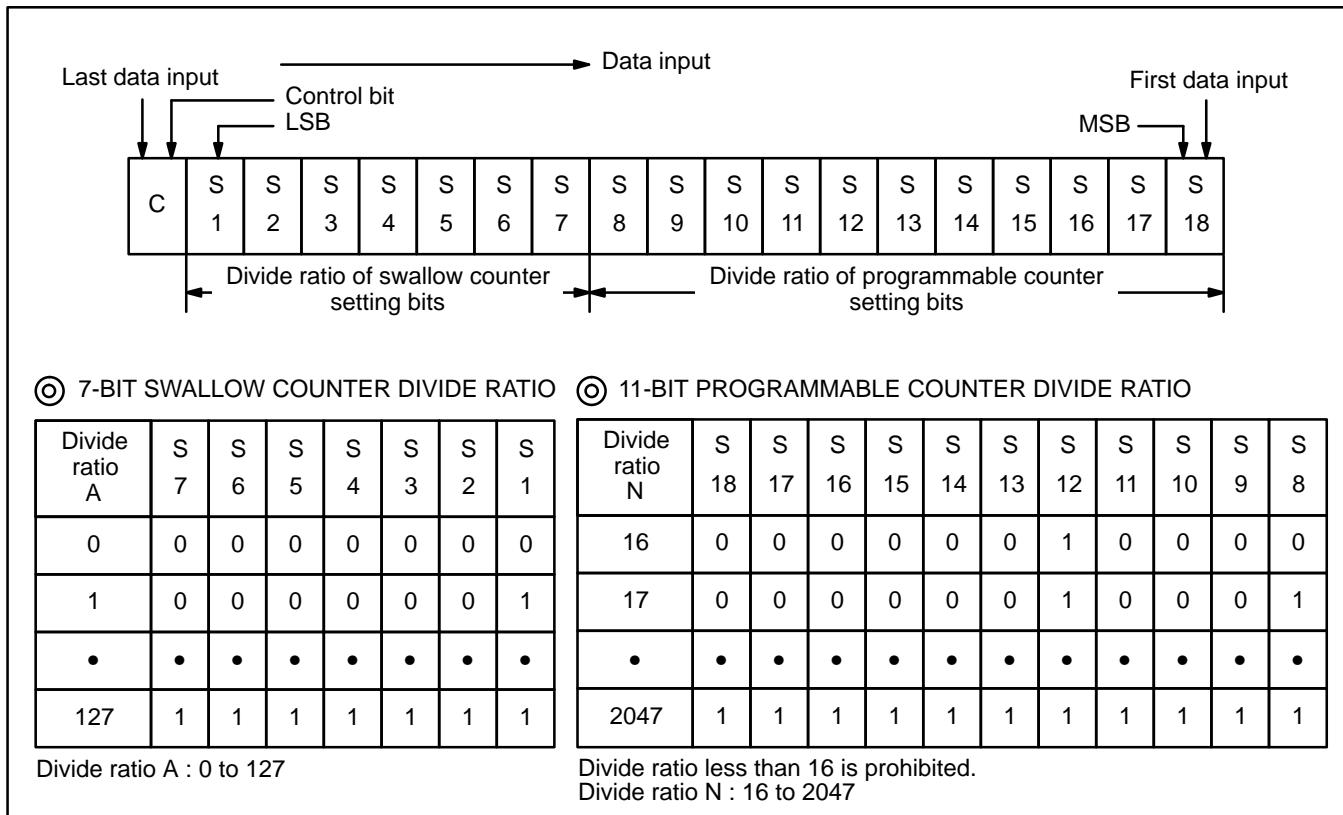
S<sub>8</sub> to S<sub>18</sub> : Divide ratio of programmable counter setting bits (16 to 2047)
