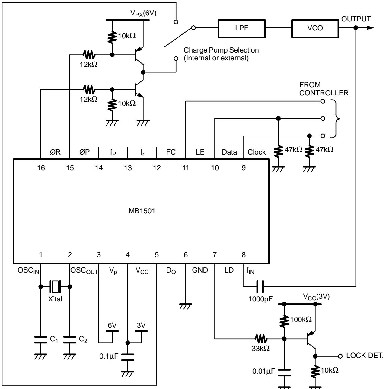
C<sub>1</sub>, C<sub>2</sub>: Depends on crystal oscillator
