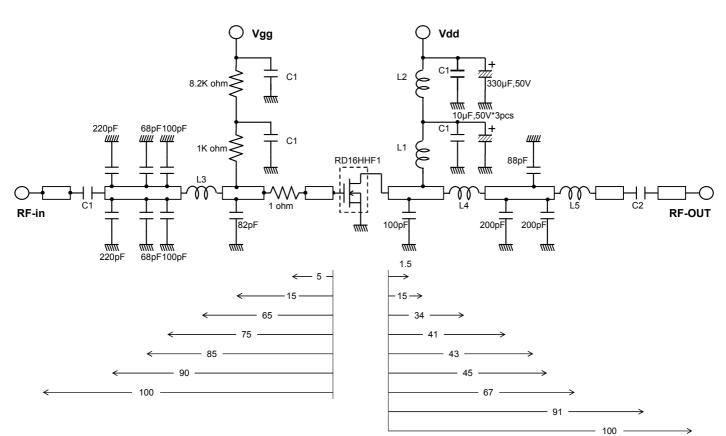
C1:100pF,0.022 $\mu$ F,0.1 $\mu$ F in parallel C2:470pF\*2 in parallel
