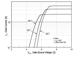
Figure 2. Transfer Characteristics
