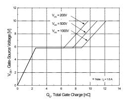
Figure 6. Gate Charge Characteristics
