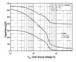
Figure 5. Capacitance Characteristics
