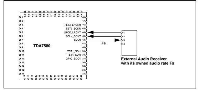
An external digital Audio device is connected externally as a digital audio master, and the internal TDA7580 Sample Rate Converter is responsible for the conversion from internal 36kHz to the external Audio Rate.
