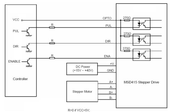
R=1K (Power > 0.125W) if VCC=12V; R=2K (Power > 0.125W) if VCC=24V; R must be connected to control signal terminal.
