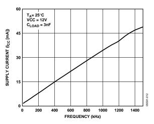
Figure 12. Supply Current vs. Frequency
