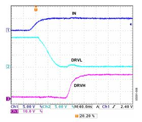
Figure 6. DRVH Rise and DRVL Fall Times  $C_{LOAD} = 6$  nF for DRVH,  $C_{LOAD} = 2$  nF for DRVH
