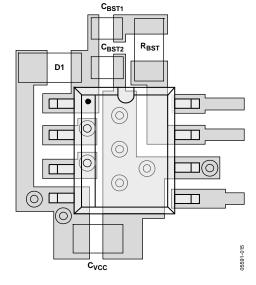
Figure 15. External Component Placement Example
