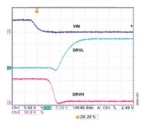
Figure 7. DRVH Fall and DRVL Rise Times  $C_{LOAD} = 6$  nF for DRVH,  $C_{LOAD} = 2$  nF for DRVH
