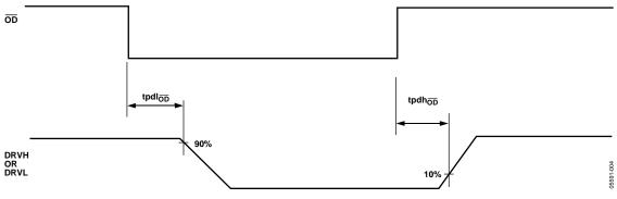
Figure 4. Output Disable Timing Diagram
