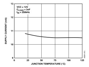
Figure 13. Supply Current vs. Temperature
