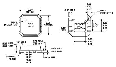
Figure 18. 8-Lead Lead Frame Chip Scale Package [LFCSP\_VD] 3 mm x 3 mm Body, Very Thin, Dual-Lead (CP-8-2) Dimensions shown in millimeters
