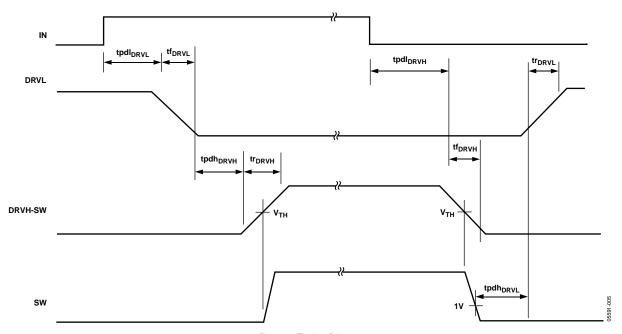
Figure 5. Timing Diagram (Timing is referenced to the 90% and 10% points, unless otherwise noted.)
