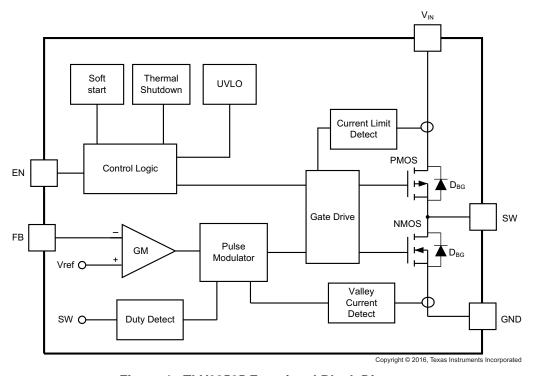
Figure 4. TLV62565 Functional Block Diagram
