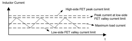
Figure 7. Switch Current Limit
