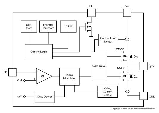
Figure 5. TLV62566 Functional Block Diagram
