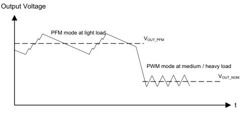
Figure 6. Output Voltage in PFM/PWM Mode
