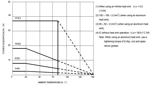
Fig.46 Power Dissipation Characteristics
