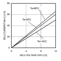
Fig.35 SEL2 Input Current
