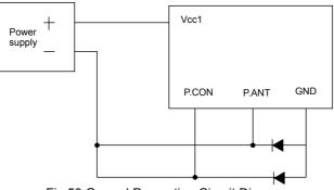
Fig.50 Ground Prevention Circuit Diagram
