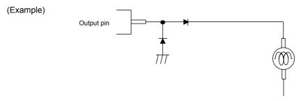
Fig.51 Example of Protective Diode Insertion
