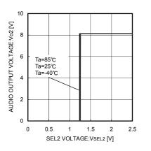
Fig.32 AUDIO Input Threshold Voltage
