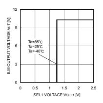
Fig.29 ILM Input Threshold Voltage
