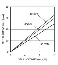
Fig.34 SEL1 Input Current
