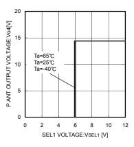
Fig.31 P.ANT Input Threshold Voltage
