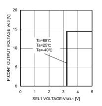
Fig.30 P.CON Input Threshold Voltage
