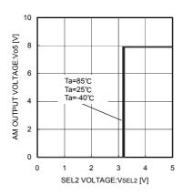
Fig.33 AM Input Threshold Voltage
