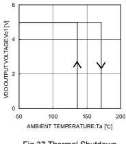
Fig.37 Thermal Shutdown Operation
