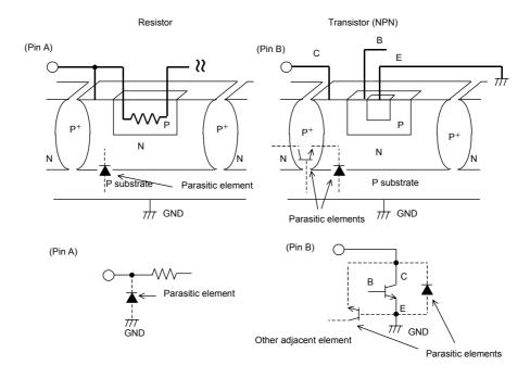
Fig.48 Example of a Simple Monolithic IC Architecture
