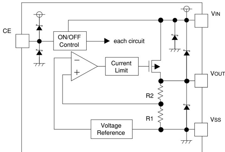
The diode in the circuit above is the protective diode.
