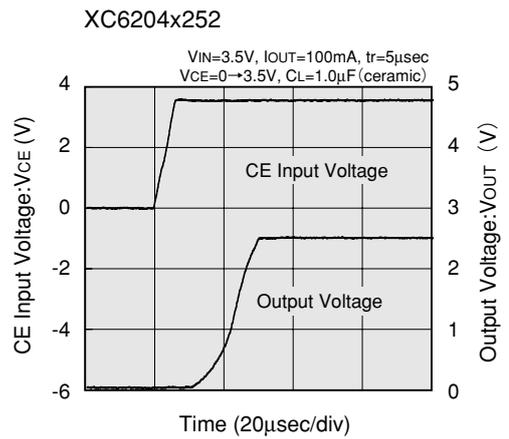
(11) ENABLE RESPONSE TIME (These characteristics will not be affected by the nature of the CE pin's logic)
