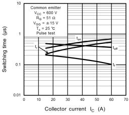
Fig. 8.8 Switching Time - I<sub>C</sub>
