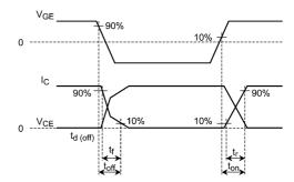
Fig. 6.2.2 Timing Chart of Switching Time
