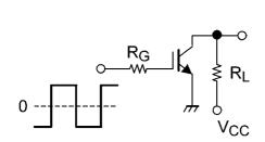
Fig. 6.2.1 Test Circuit of Switching Time
