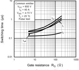
Fig. 8.7 Switching Time - R<sub>G</sub>
