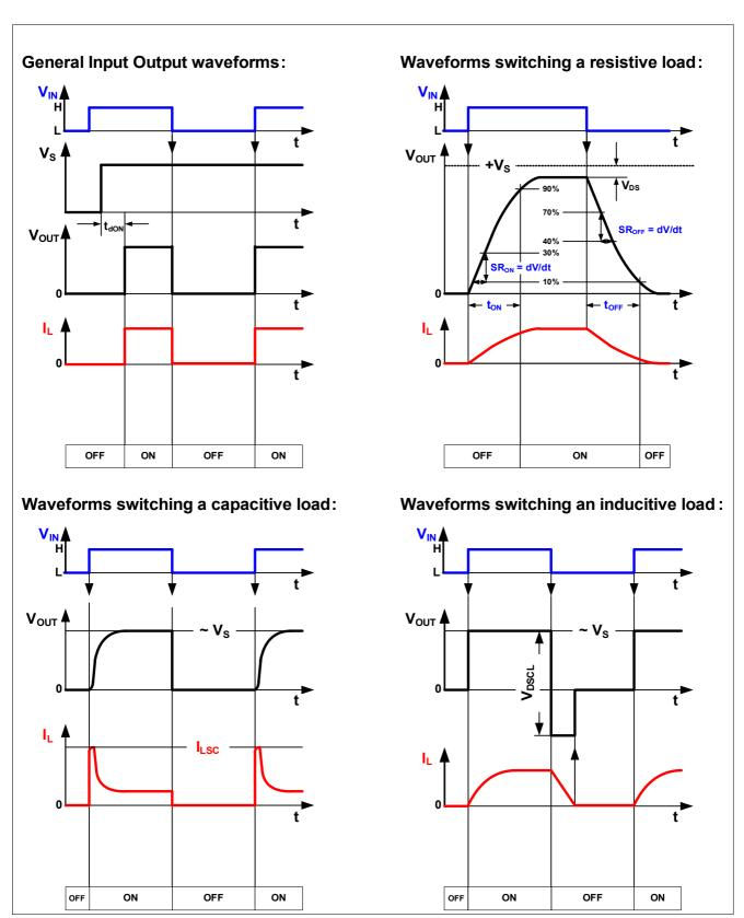
Figure 6 Typical application waveforms of the ITS4200S-ME-P
