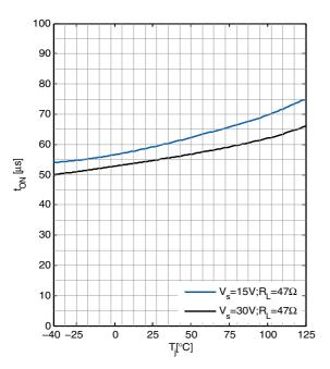
ON Slewrate  $SR_{ON}$  versus Junction Temperature  $T_{i}$
