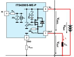
When an inductive load is switched off a current path must be established until the current is sloped down to zero (all energy removed from the inductive load). For that purpose the series combination  $Z_{\text{DSCL}}$  is connected between Gate and Drain of the power DMOS acting as an active clamp.
