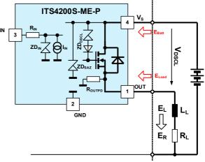
Energy stored in the load inductance is given by :  $E_1 = I_1^{2*}L/2$
