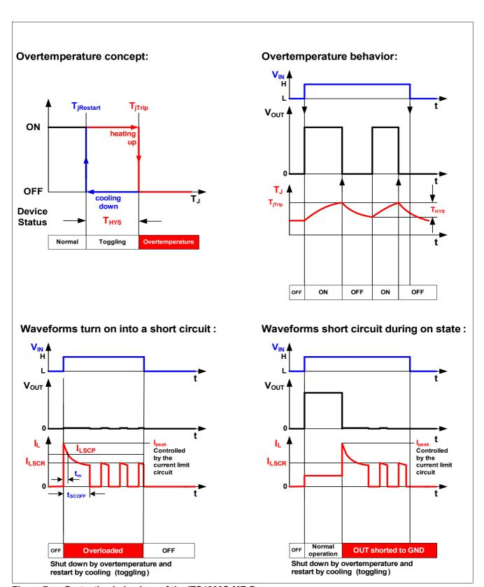
Figure 7 Protective behaviour of the ITS4200S-ME-P
