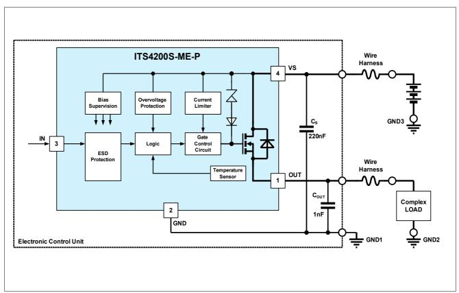
Figure 4 Application Diagram
