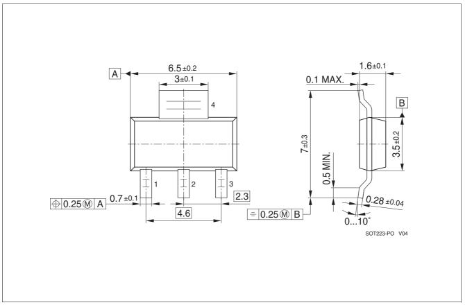
Figure 8 SOT-223-4 (Plastic Dual Small Outline Package, RoHS-Compliant)
