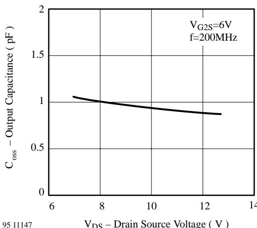
Figure 6. Output Capacitance vs. Drain Source Voltage
