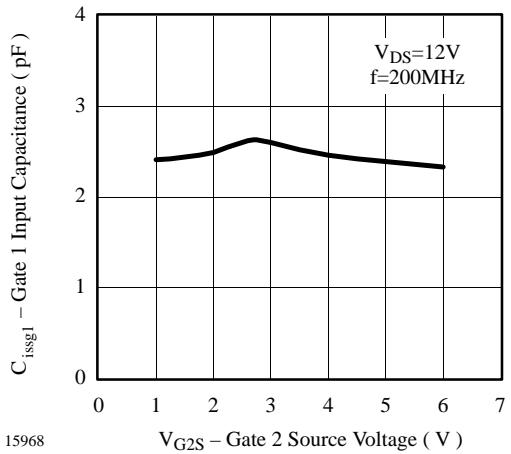
Figure 5. Gate 1 Input Capacitance vs.
