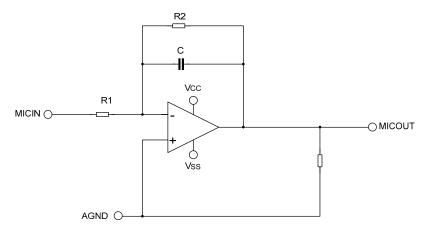
The proportional amplifier shown as above is adopted for microphone amplifier with setting gain of about 29dB, and capacitor C is used for high frequency signal filtering. As described above, the gain can be also adjusted by changing R1.
