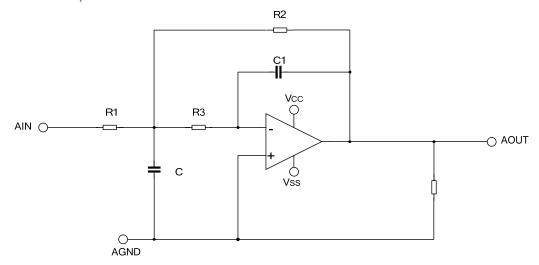
The second-order filter structure shown as above is adopted for 6-channel audio amplifier, with in-band gain of about 12dB and -3dB bandwidth of 40kHz above which is well meet audio requirements. As principle structure, in-band gain is decided by:  $G = -\frac{R_2}{R_1}, \text{ thus, gain can be adjusted by changing R1.}$
