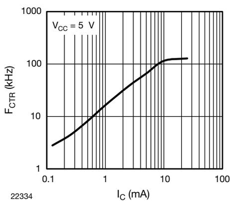
Fig. 14 -  $F_{CTR}$  vs.  $I_C$  (sat) (mA)
