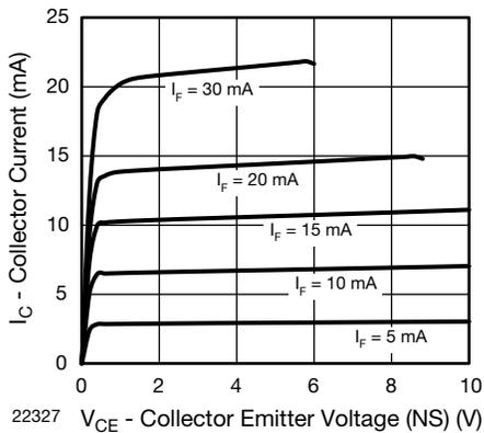
Fig. 7 - Collector Current vs. Collector Emitter Voltage (NS)
