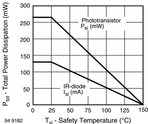
Fig. 1 - Derating Diagram
