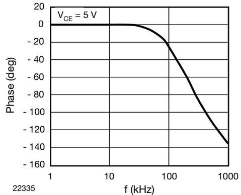
Fig. 15 -  $F_{CTR}$  vs. Phase Angle (kHz)
