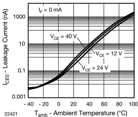
Fig. 8 - Leakage Current vs. Ambient Temperature
