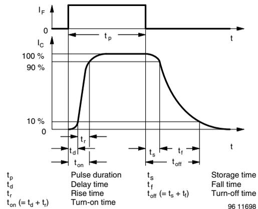
Fig. 5 - Switching Times
