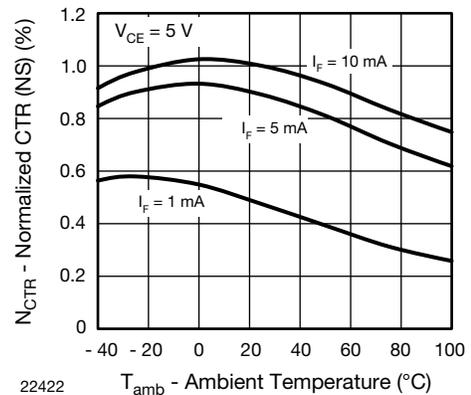
Fig. 11 - Normalized CTR (NS) vs. Ambient Temperature
