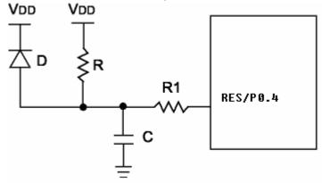
External Power-On Reset circuit is required only if VDD power-up is too slow. The diode D helps discharge the capacitor quickly when VDD powers down.
