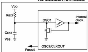
The oscillator frequency, when in EXT RC, divided by 4, is available on the OSCOUT/P0.6 pin, and can be used for test purposes
