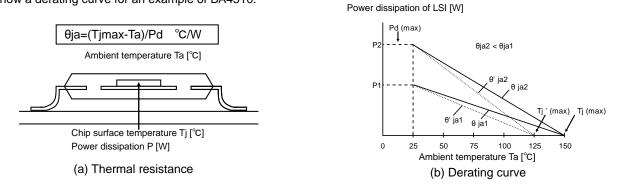
Figure 29. Thermal resistance and derating curve
