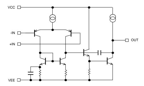
Figure 1. Simplified schematic
