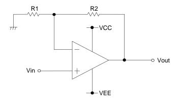
Figure 33. Non-inverting amplifier circuit
