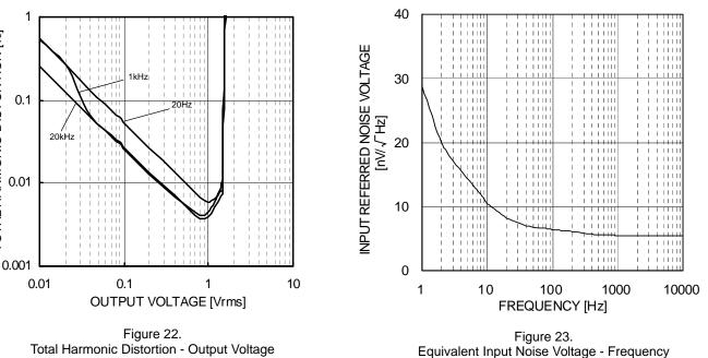
(VCC/VEE=2.5V/-2.5V, RL=3k $\Omega$ , 80kHz-LPF, Ta=25°C)
