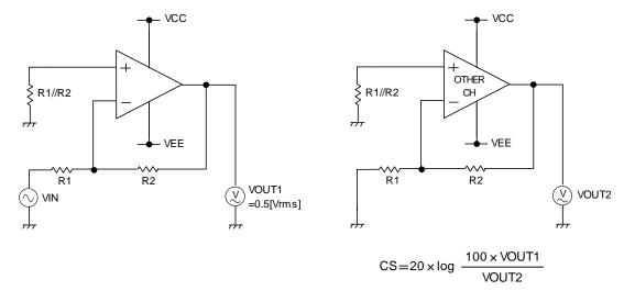
Figure 28. Test Circuit 3 (Channel Separation) (VCC=+2.5V. VEE=-2.5V, R1=100Ω, R2=10kΩ)
