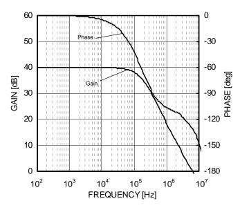
Figure 24. Voltage Gain • Phase - Frequency (VCC/VEE=2.5V/-2.5V, Av=40dB, RL=10kΩ)
