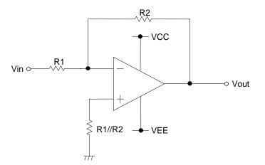
Figure 32. Inverting amplifier circuit
