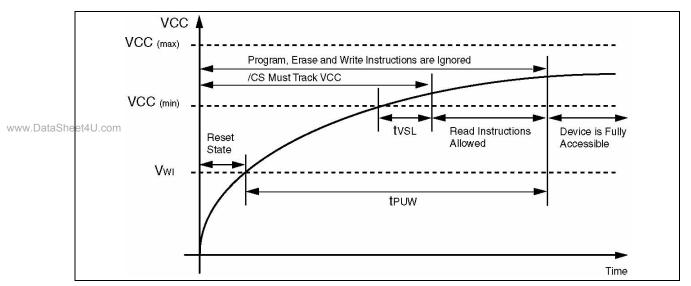
Figure 20. Power-up Timing and Voltage Levels
