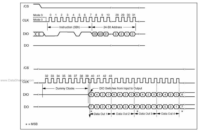
Figure 10. Fast Read Dual Output Instruction Sequence Diagram
