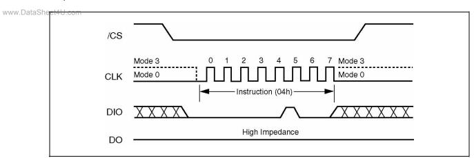
Figure 5. Write Disable Instruction Sequence Diagram
