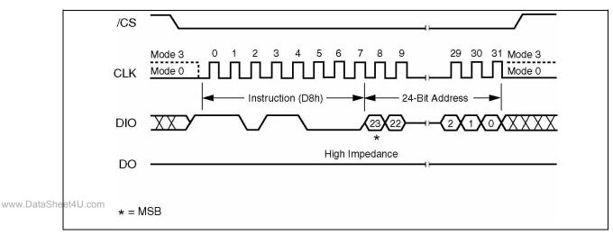
Figure 13. Block Erase Instruction Sequence Diagram
