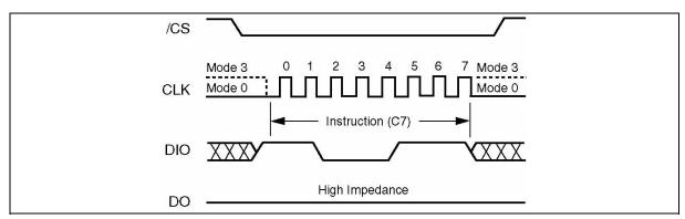
Figure 14. Chip Erase Instruction Sequence Diagram
