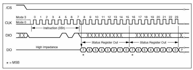
Figure 6. Read Status Register Instruction Sequence Diagram
