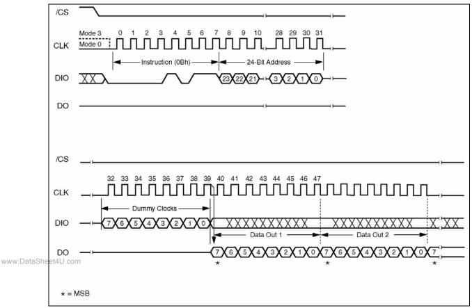
Figure 9. Fast Read Instruction Sequence Diagram
