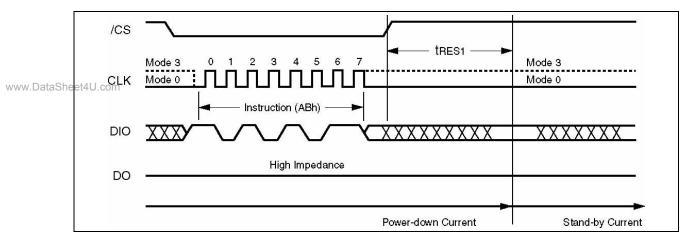
Figure 16. Release Power-down Instruction Sequence
