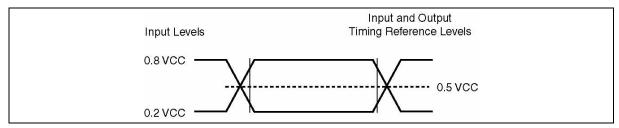
Figure 21. AC Measurement I/O Waveform
