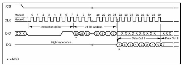
Figure 8. Read Data Instruction Sequence Diagram
