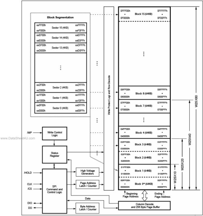
Figure 2. W25X10, W25X20, W25X40 and W25X80 Block Diagram
