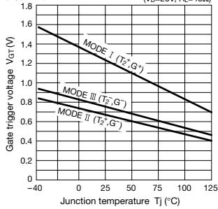
$i_{GT}$  temperature characteristics (Typical) ( $V_D = 20\text{V}$ ,  $R_L = 40\Omega$ )
