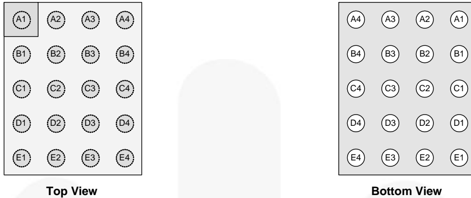
Figure 3. WLCSP-20 Pin Assignments
