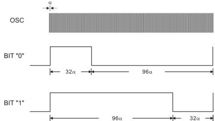
where the oscillating time period,  $\alpha = 1/f$  and (f is the oscillation frequency)
