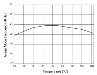
Fig. 4 Green Mode Frequency vs. Temperature
