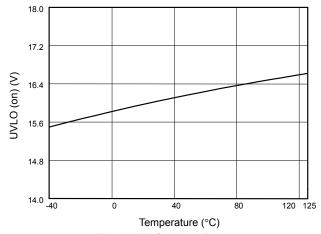
Fig. 1 UVLO (on) vs. Temperature
