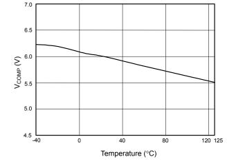
Fig. 11 V<sub>COMP</sub> open loop voltage vs. Temperature
