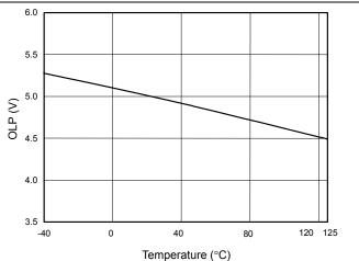
Fig. 12 OLP-Trip Level vs. Temperature
