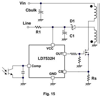
A 220nS leading-edge blanking (LEB) time is included in the input of CS pin to prevent the false-trigger caused by the current spike. In a low power application, if the total pulse width of the turn-on spikes is less than 220nS and the negative spike on the CS pin doesn't exceed -0.3V, the R-C filter as shown in the figure16 could be eliminated.
