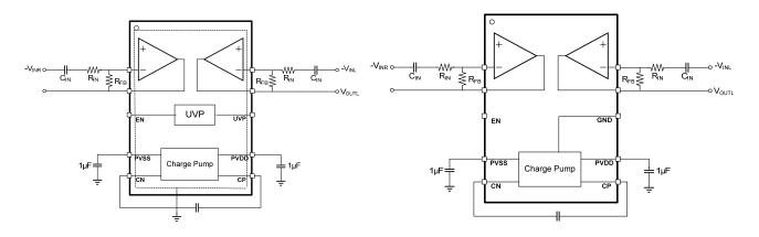
Figure 3 Typical Application Circuit of TPF605 (Left) and TPF607 (Right)
