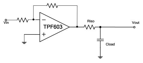
Figure 8 Driving Circuits
