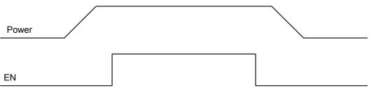
Figure 6 The Sequence of EN Control
