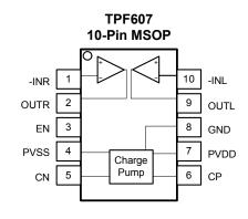
3-V<sub>RMS</sub> Audio Line Driver with Integrated Charge Pump
