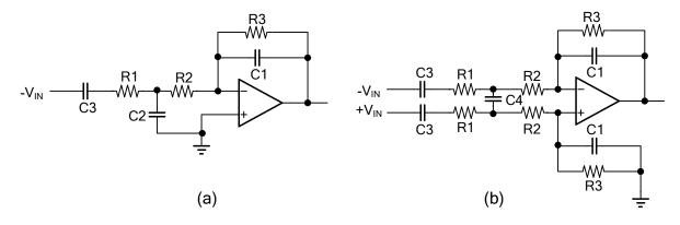
Figure 5 Second-order filter with gain: (a) Single-ended input; (b) Differential input
