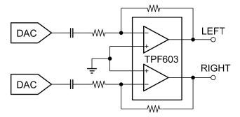
Figure 1. Typical Application Circuit of TPF603
