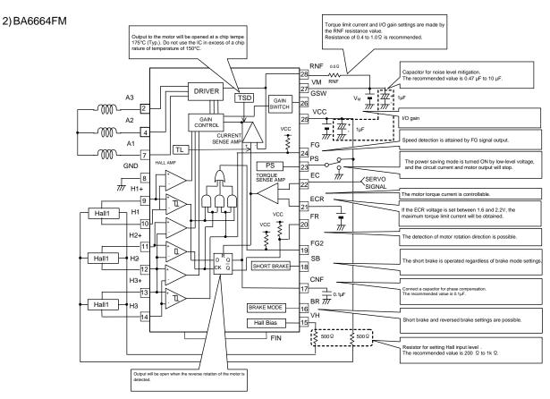
Fig.6 BA6664FM Block Diagram
