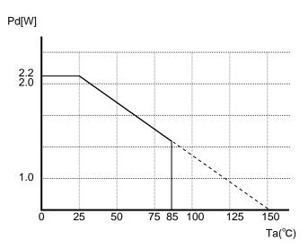
Fig.7 Power Dissipation Reduction (BA6664FM、BD6671FM)
