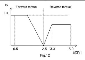
The relation between the input gain and torque limit current expressed as (1) and (2) discussed previously is only valid when EC and ECR are within a range from 0.5V to 3.3V. Depending on how the torque control reference terminal voltage, ECR is specified, there may be a case when the output current for the motor does not go up to the torque limit value. Please be aware of this voltage range when specifying the ECR voltage.
