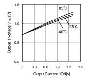
Fig.2 Output Saturation Voltage at High Level
