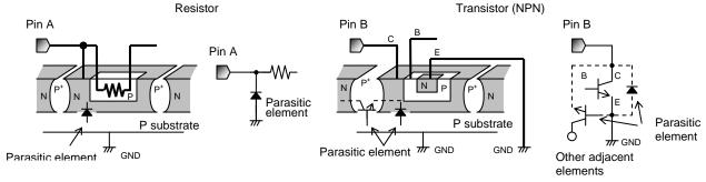
Fig.18 Example of IC structure
