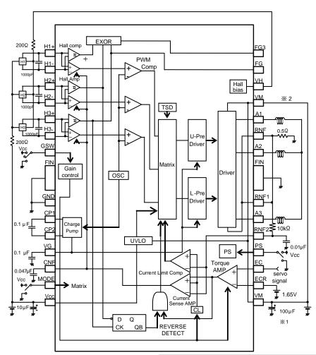
X 1 Set capacitor between VM and GND, close as possible to the IC.X2 To prevent from concentration of current routes, make the wiring impedance values from the power supply equal as possible.
