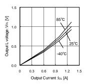
Fig.3 Output Saturation Voltage at Low Level
