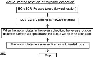
Fig. 13 shows the construction of the reverse rotation detection circuit.
