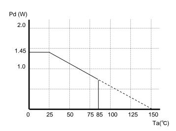
Fig.5 Power Dissipation Reduction (BA6859AFP-Y)
