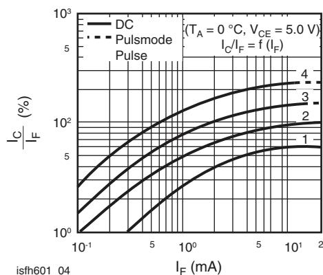
Fig. 4 - Current Transfer Ratio vs. Diode Current
