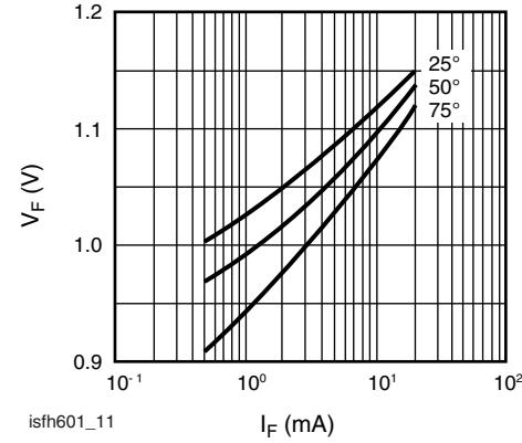
Fig. 11 - Forward Voltage
