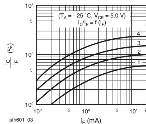
Fig. 3 - Current Transfer Ratio vs. Diode Current
