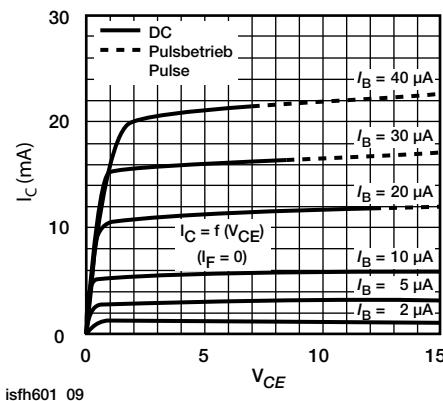
Fig. 9 - Transistor Characteristics
