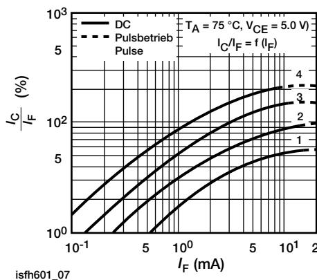
Fig. 7 - Current Transfer Ratio vs. Diode Current
