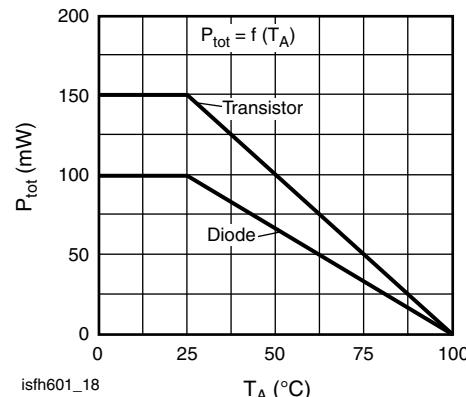
Fig. 18 - Permissible Power Dissipation for Transistor and Diode
