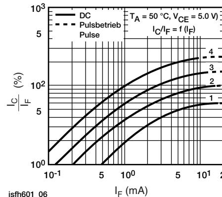
Fig. 6 - Current Transfer Ratio vs. Diode Current
