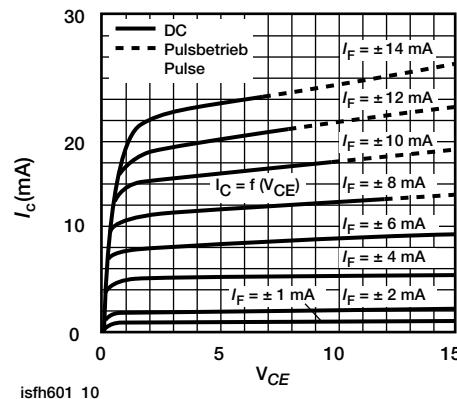
Fig. 10 - Output Characteristics
