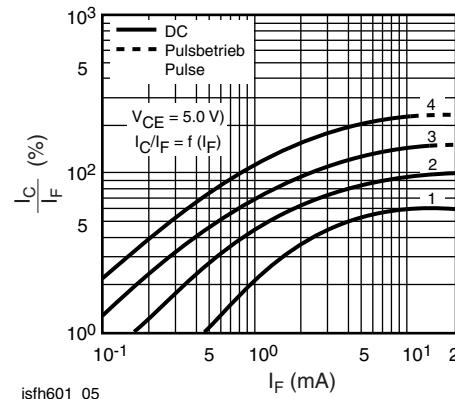
Fig. 5 - Current Transfer Ratio vs. Diode Current
