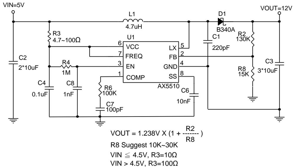
(4) **FREQ=Low (Frequency=680KHz) (SOP-8L/MSOP-8L)**
