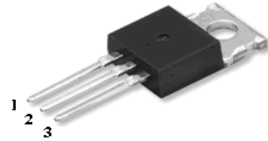
1. Gate 2. Drain 3. Source
