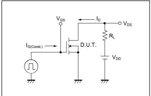
Fig.3-1 Avalanche Measurement Circuit
