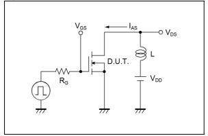
Fig.4-1 trr Measurement Circuit
