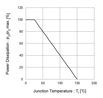
Fig.2 Drain Current Derating Curve
