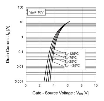
Fig.10 Gate Threshold Voltage vs.
