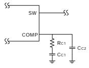
With current mode, the buck power stage can be simplified to be a 1 pole and 1 zero. The compensation network provides 2 poles and 1 zero. They are determined by the following formulas:
