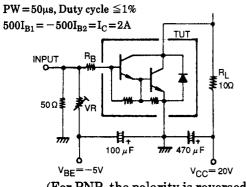
(For PNP, the polarity is reversed.) Unit (resistance :  $\Omega$ , capacitance : F)
